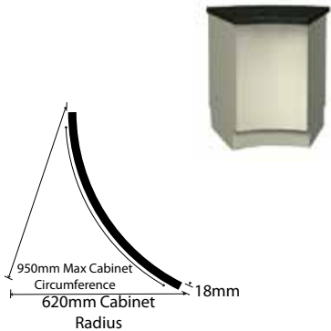
19b Concave Curved Mould Maximum Height = 1000mm 620R Max door width = 950mm
