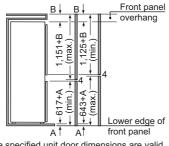
The specified unit door dimensions are valid for a door gap of 4 mm. If a different gap width is used (max. 14 mm), the dimensions must be adjusted.
