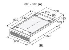
A: Area for cable outlet on the ceiling B: Front of appliance
