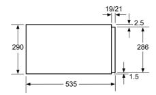
Ovens with an appliance height of 595 mm can be installed above a warming drawer.
