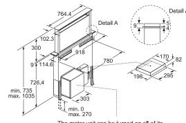
The motor unit can be turned on all of its four sides, fitted on the front or the rear or offset at a distance from the appliance. (Special accessory required)
