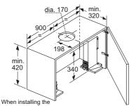
90 cm telescopic hood in a 90 cm wide wall-hanging cupboard, the mounting kit is required. The two mounting brackets are screwed onto the right and left of the kitchen unit. Installation in accordance with template.
