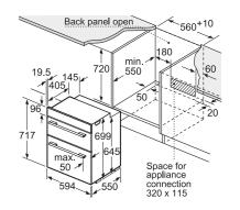
If the appliance will be installed underneath a hob, the following worktop thicknesses (including substructure if necessary) must be taken into account.
