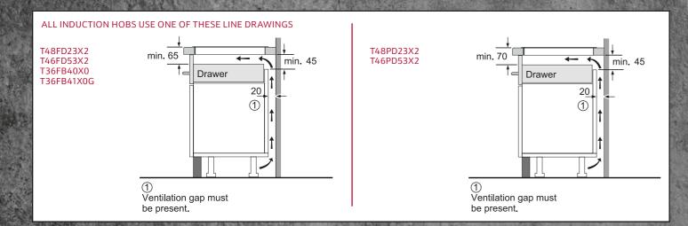
ALL INDUCTION HOBS USE THESE LINE DRAWINGS T48PD23X2, T46PD53X2, T48FD23X2, T46FD53X2, T36FB40X0, T36FB41X0G - 5 Built-in cooker/ ① Ventilation gap must be present
