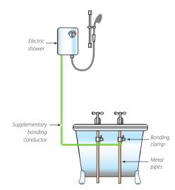
Bonding is used to reduce the risk of electric shocks to anyone who may touch two separate metal parts when there is a fault somewhere in the supply or electrical installation. By connecting bonding conductors between particular parts, it reduces the voltage there might have been.
